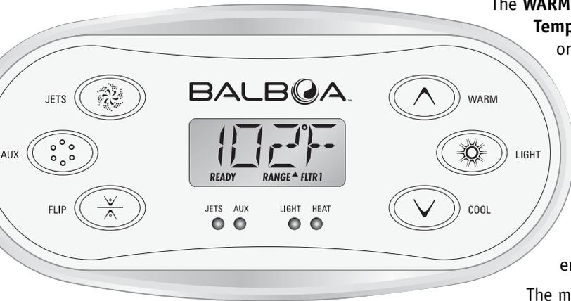
The **WARM** and **COOL** buttons are indicated by a single **Temperature** icon throughout this User Guide. Some panels only have one Temperature Button.
